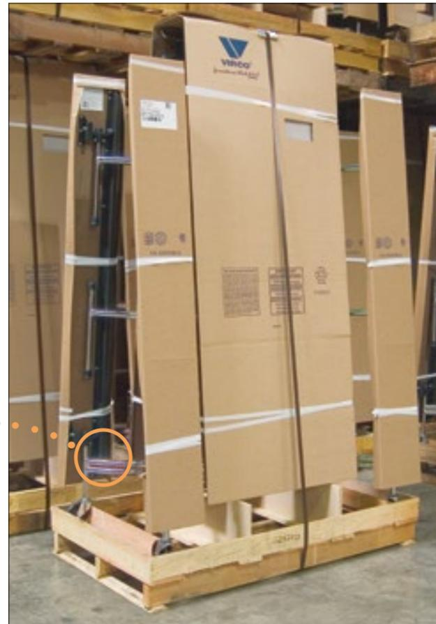
Protective cardboard and banding to the pallet minimize freight damage.
