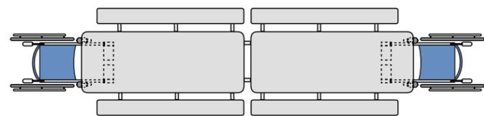
Rectangular mobile bench and mobile stool tables are ADA compliant and are designed to accommodate one wheelchair at either end.
