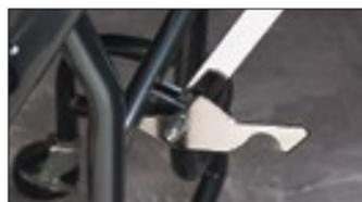
An up-lock mechanism holds tables in place while folded, and a down-lock mechanism holds tables in place when unfolded.
